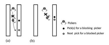
**Fig. 2.** Types of picker blocking: (a) in-the-aisle (picker) blocking and (b) pick-point blocking (Parikh and Meller, 2009).
