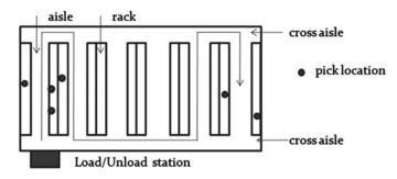
**Fig. 1.** A typical parallel-aisle OPS and a routing example (modified from Gademann and Van de Velde (2005)).
